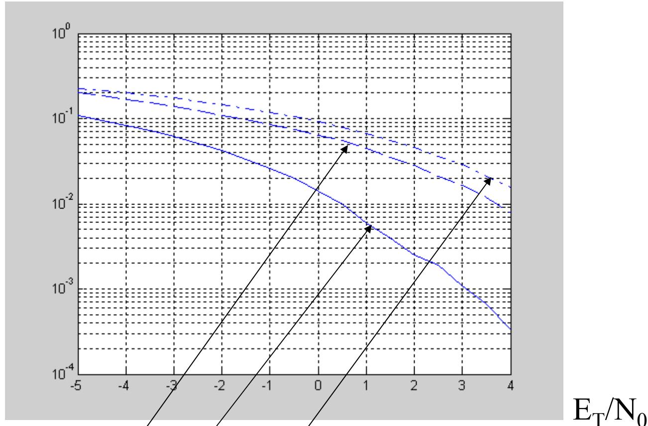
BER versus SNR for a MIMO system without CSIT. De abajo a arriba; MIMO(4,4) six streams and four PCUs ( $r=3/4$ ); MIMO(3,3); MIMO(2,2) four streams and 2 PCUs ( $r=1$ ).
