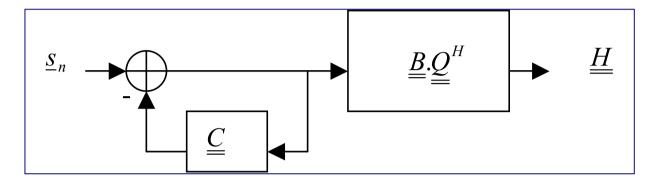
Note that matrix Q does not destroys the optimallity of B, since it id orthonormal, but the inverse of I+C does. In fact the recursive scheme, in addition to a non-diagonal character, introduces diagonal values which are greater than one.
