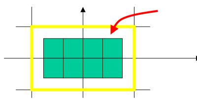
Thresholds for modulus operation on a 8QAM constellation
