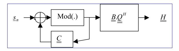
The modulus operation have to be introduced independently For in-phase and quadrature components of the constellation
