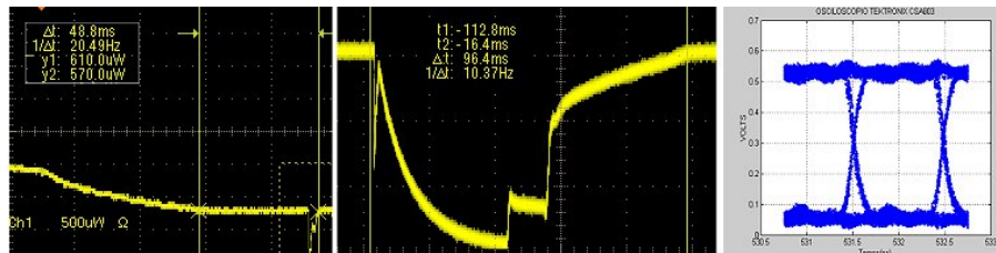
Figure 1: Service unavailability (left, recovery with degraded SLA, middle, full recovery) in power/time and example of BER measurement at 1 Gbps (right).
